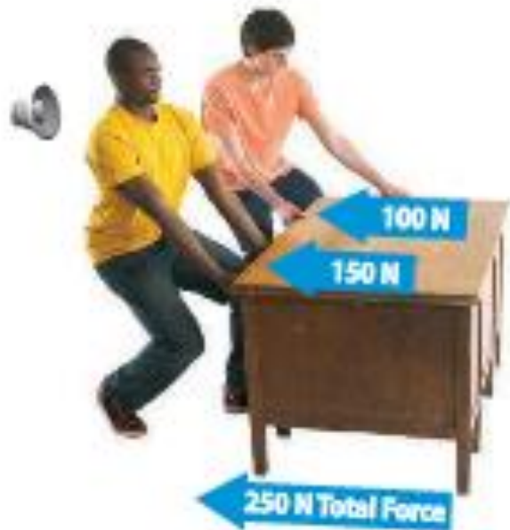
Figure 6 The net force acting on an object is the sum of the two forces and acts in the same direction.
